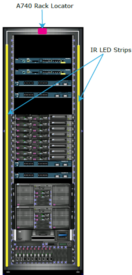
Figure 13: LED Strips and A740 Rack Locator Positioning in Rack
