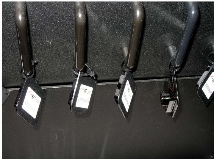
Figure 20: R114 Rack Tag Mounted with Lens Pointing Downward
