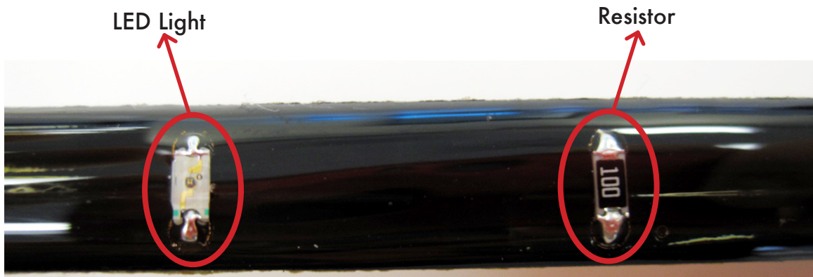
Figure 13: LED Light and Resistor in the LED Strip
