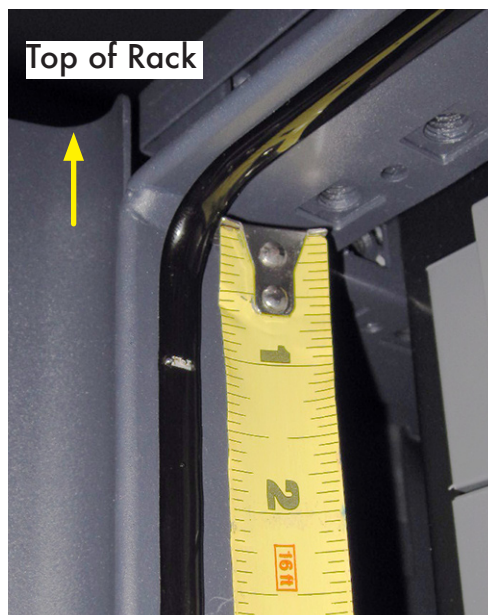
Figure 15: Application of First LED Strip to Top of Rack
