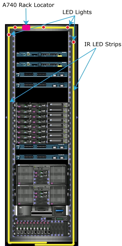
Figure 14: LED Strips and A740 Rack Locator Positioning in Rack
