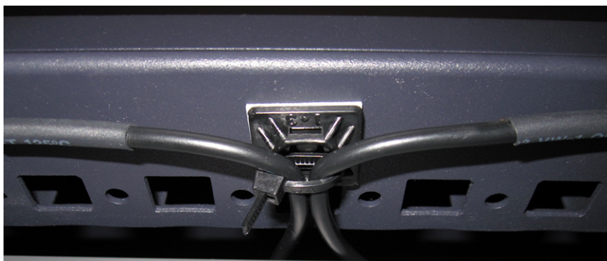
Figure 18: Tie Wrapped Connector Wires
